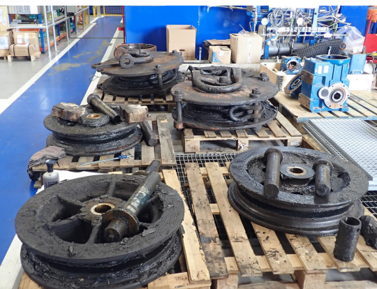
Worn pulleys at Plymouth Service Centre
