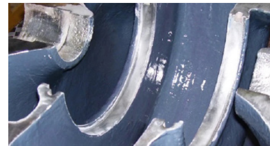
Finished casing with wear resistant coating
