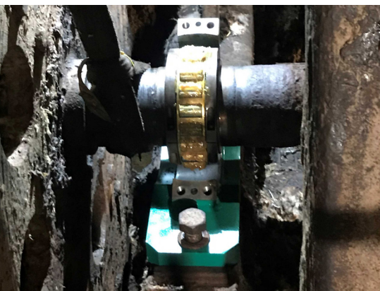
Support cap and housing removed exposing internal components
