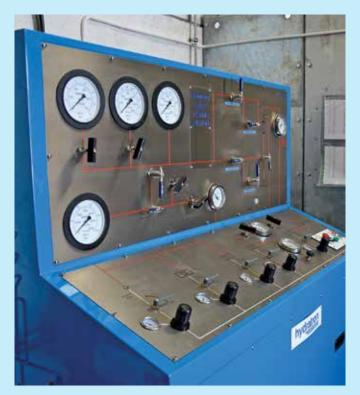
High volume - High pressure gas: 10,000psi gaseous media Hydro-testing up to pressure class 300 Hydro-testing up to pressure class 2500 Nitrogen Gas (N<sub>o</sub>) Test media system -Ambient temperature gas testing up to pressure class 2500
