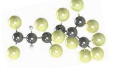
FKMs (sometimes known as FPMs in Europe) are frequently used to resist extreme temperatures and harsh chemicals. The strong carbon-fluorine bonds that make up the polymer structure provide high thermo-chemical resistance, giving excellent ageing characteristics shown by low compression set at elevated temperatures.
