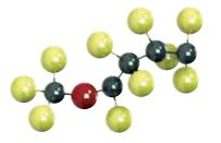
Perfluoroelastomers (FFKM) have a fully fluorinated polymer backbone resulting in a fluorine content >71%. As the material is free from carbon-hydrogen bonds in the polymer chain, the FFKM materials offer the ultimate thermo-chemical resistance.
