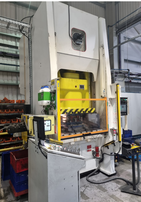
Upgraded press with mobile filtration unit (MFU) in situ
