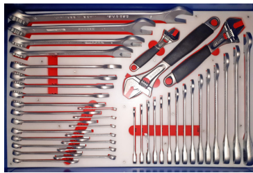
New situation: Plastic inlay according to EC1935/2004 for High Care Zone
