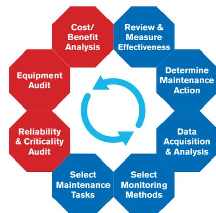
The steps in the red highlighted sections need to be in place before a CM provider considers making changes to an organisation's maintenance regime. Without this data – and measurable uptime, availability, energy and throughput data – there is no benchmarking and therefore it will not be possible to measure improvements or return on investment.
