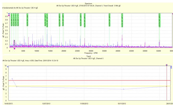
Vibration spectral and overall data before and after investigation and repair
