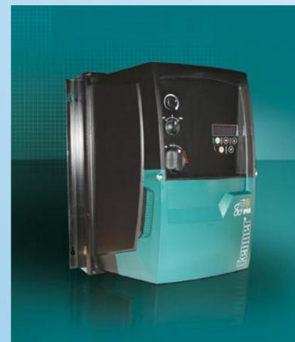
The Fenner QuickDrive (QD) range of inverters is being expanded with the addition of an IP66 rated QD:E model. The IP66 unit is available from 0.37kW to 7.5kW (110-440V) and is specifically designed with a smooth crevice free shape to reduce the opportunities for the build-up of debris. The Fenner QD:E (E for Easy) selection of drives are competitively priced, with pre-set factory settings that
