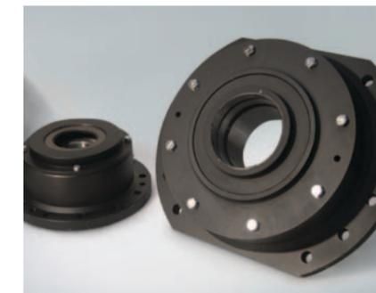
ingress of contaminants. The assemblies are pre-greased and ready to fit, with bearing location features and provision for re-greasing. The series of spherical roller bearings used are designed specifically to provide improved bearing life under severe operating conditions, and can reduce levels of both vibration and noise by 50–60%.
