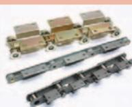
This chain is used extensively in the conveying of bulk food stuffs such as grain, maize, wheat and raw food mixtures and waste processing by-products. Most of these applications use scraper type conveyor systems that normally have long centre distances between sprockets. Such systems are sometimes slow moving with little or no shock loading, hence the chain has to take the strain.
